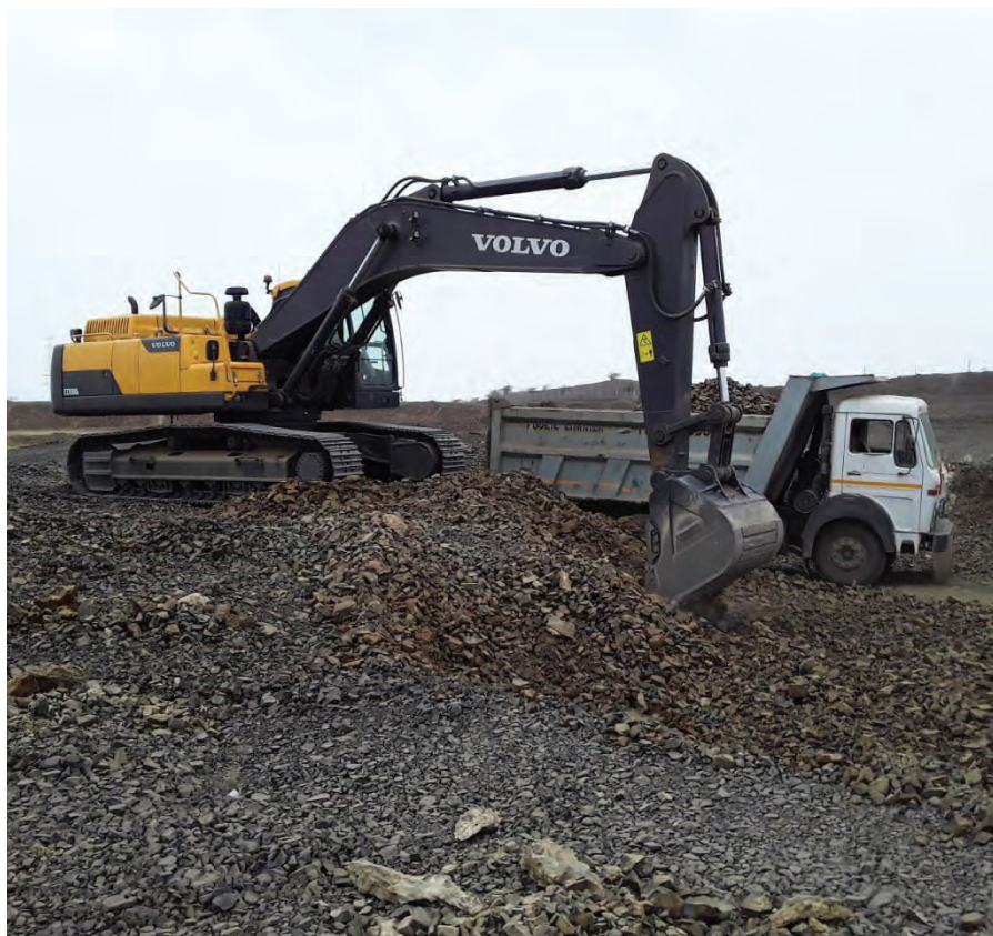
ABOVE AND BELOW: The Volvo EC350D crawler excavator being deployed in a stone quarry located in the district of Kachchh, at a site known as Vidi in Anjar Taluka. The machine works on demanding applications such as excavating and loading stones on to the tippers.
