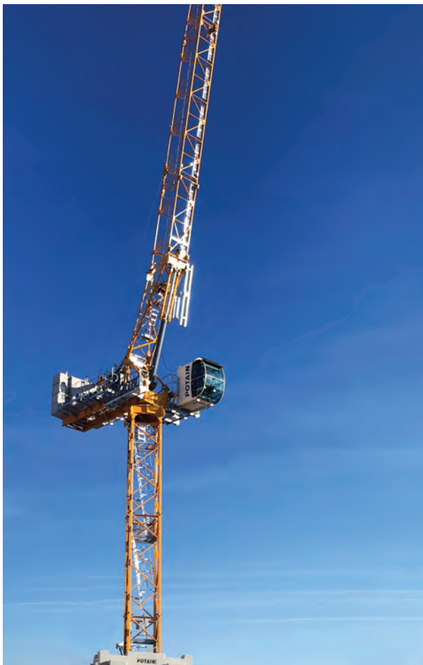
The new Potain MRH 175 hydraulic luffing jib crane offers a maximum capacity of 10 t, while its maximum jib length is 55 m.
