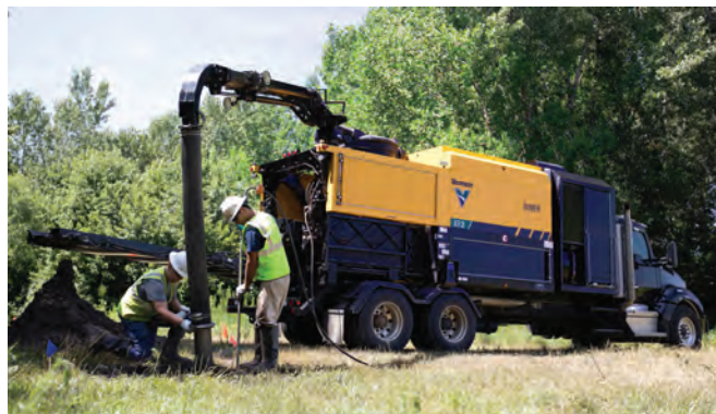
ABOVE AND LEFT: Vermeer XR2 vacuum excavator is equipped with a shaker deck that separates liquids and solids to allow contractors to stay on the jobsite longer, work efficiently and reduce disposal expenses.
