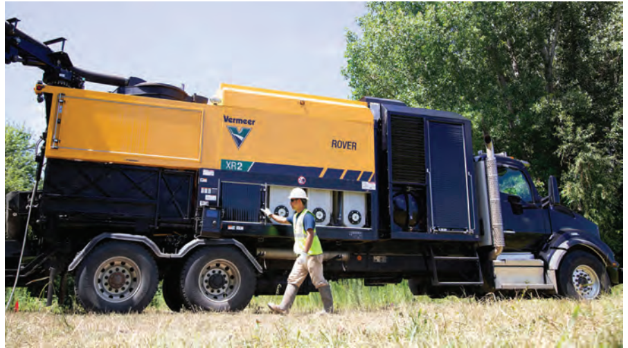
ABOVE AND LEFT: Vermeer XR2 vacuum excavator is equipped with a shaker deck that separates liquids and solids to allow contractors to stay on the jobsite longer, work efficiently and reduce disposal expenses.
